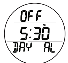
Fig. 20 - DAILY ALARM STATUS (to access Set)
